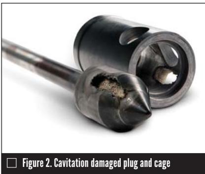
□ Figure 2. Cavitation damaged plug and cage
