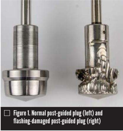
□ Figure 1. Normal post-guided plug (left) and flashing-damaged post-guided plug (right)
