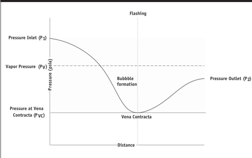
□ Figure 6. Pressure profile showing how cavitation occurs
