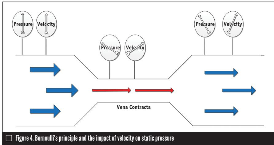
□ Figure 4. Bernoulli's principle and the impact of velocity on static pressure
