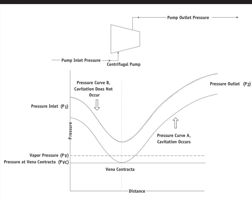
ensure the pump does not cavitate, as shown in curve B. In this case, the pressure at the eye of the impeller still drops below the inlet suction pressure of the pump, but the pressure of the liquid at the eye of the impeller remains above the liquid vapor pressure so no cavitation occurs.
