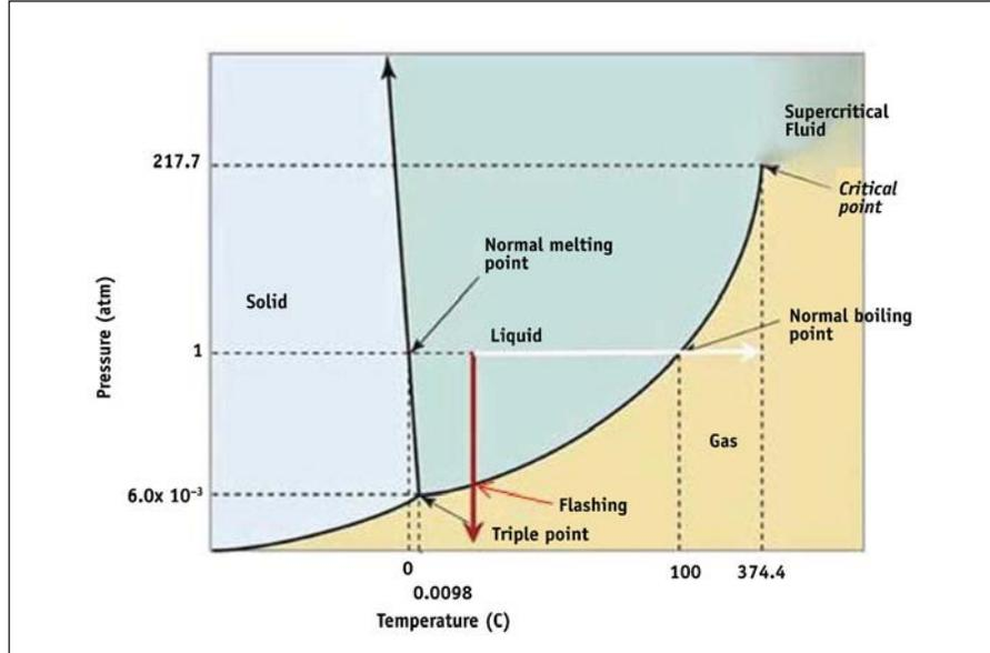
□ Figure 3. Phase diagram showing boiling and flashing (Machado, 2009)
