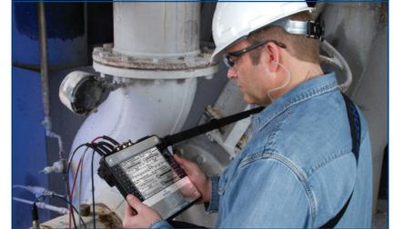
**Emerson’s CSI 2140 Machinery Health Analyzer is best-in-class for speed and performance in field vibration data collection and analysis.**
