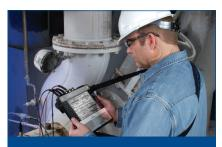
Emerson's CSI 2140 Machinery Health Analyzer is best-in-class for speed and performance in field vibration data collection and analysis.
